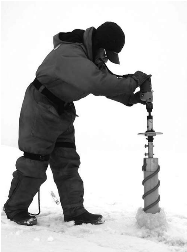
A wildlife observer from the Department of Fisheries and Oceans Canada drills through the pack ice. The ice core was analyzed and the water samples collected from the hole left in the ice.
