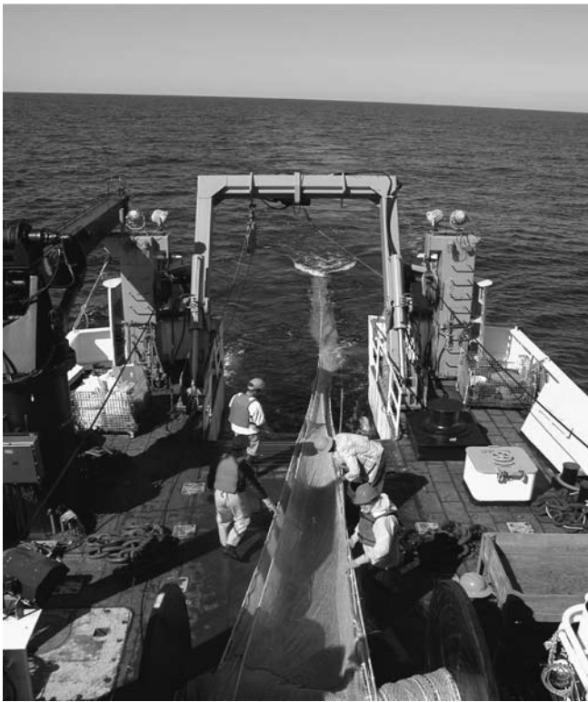
Midwater trawl coming on board the fisheries research vessel Delaware II. The trawl catch is used to verify the species composition of acoustic backscatter and for biological information such as fish length, weight, maturity, age, sex, and diet.
