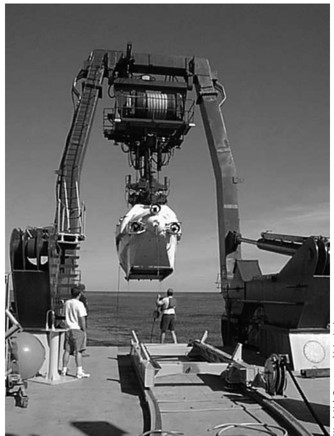
The Alvin , a US Navy deep submergence vehicle, is deployed via the A-frame crane off the stern of the US Navy's research vessel Atlantis .
