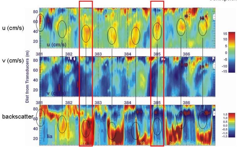
Bacscatter periodic variations seem out of phase with internal wave propagation.
